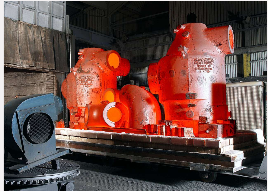
Steel castings after undergoing 12-hour 1,200 °C (2,190 °F) heat treatment.
