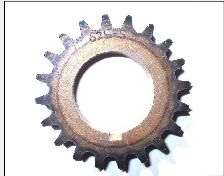
A flame-hardened sprocket. The discoloration around the teeth delineates the area that was rapidly heated and then quenched.
